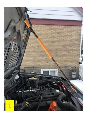
6. Prop the hood in the chosen open position using a 2"x4" cut to length, an extension pole, or other suitable means (**Fig 1**). It is recommended that a prop tool be used instead of relying on a helper to hold the hood, because it is important to have the hood stay in the same position throughout the installation process.
