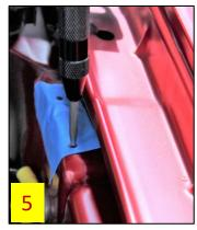
9. Install a #9 indexed or 3/16" drill bit into a drill, and place the included drill bit stopper next to the drill bit (note - #9 drill bit is preferred and is available on our website). Mark the stopper with a permanent marker about 3/8" short of the drill bit tip (**Fig 6**), then cut the stopper with a utility knife at that location. Slip the drill bit stopper over the drill bit, confirm that no more than ~3/8" is protruding (**Fig 7**). This will limit the drill bit's reach during drilling.
