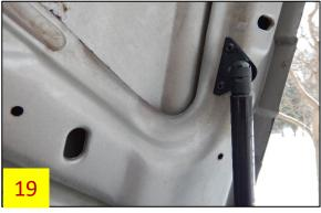
23. Repeat steps 15 through 22 for the passenger side. Do NOT assume that the location of the passenger side hood bracket will be identical to the driver side. Instead of measuring, use the same procedure for installing the bracket on the passenger side as you did for the driver side.
