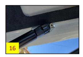
23. Remove the strut from the flat bracket to gain access for drilling the second hole. To disconnect the strut from the bracket, use a flat blade screwdriver to lift the semi-circular clip at the back of the fitting, until the fitting can be removed from the bracket (**Fig 17**). Do not fully remove the clip.
