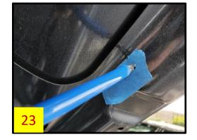
23. Line up the bracket hole with the drilled hole, and use a 3/16" rivet to attach the bracket (**Fig 24**). You may have to remove the strut from the bracket to gain access for rivet installation (see Step 30).
