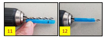
11. Drill two holes at the marked locations through the inner fender, using a slow speed and steady pressure on the bit (**Fig 13**). Apply WD-40 as needed to cool the bit. Remove the tape. Touch up the drilled holes with primer and paint.
