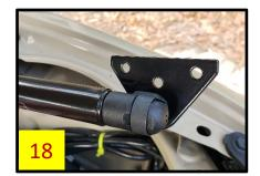
18. Raise the strut and flat bracket up until the bracket meets the inner side of the hood reinforcement (facing the center of the truck, NOT the outside) (**Fig 19 & 20**). The bracket should be just below the inside corner, flat against the reinforcement.
