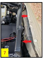
8. Apply painter's tape to the driver side inner fender edge, centered over the rear V-indentation as shown by red arrow (**Fig 8**). Place one 90 deg bracket over the tape, centered over the indentation (**Fig 9**).
