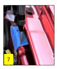
9. Install a #9 indexed or 3/16" drill bit into a drill, and place the included drill bit stopper next to the drill bit (note - #9 drill bit is preferred and is available on our website). Mark the stopper with a permanent marker about 3/8" short of the drill bit tip (**Fig 8**), then cut the stopper with a utility knife at that location. Slip the drill bit stopper over the drill bit, confirm that no more than ~3/8" is protruding (**Fig 9**). This will limit the drill bit's reach during drilling.
