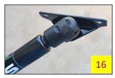
19. Raise the strut and bracket up until the bracket meets the bottom of the hood reinforcement as shown in **Fig 17**. The bracket should be centered on the bottom of the reinforcement.
