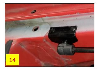
**NOTE**: Do **NOT** push the tube end fitting of the strut (with the SPIKER sticker) onto the fender ball bracket. See **Fig 15** for correct strut orientation.
