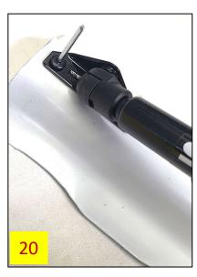
24. Adjust the bracket to be parallel with the hood reinforcement. Using the bracket as a guide, drill the second hole and install the second rivet to complete the bracket installation (**Fig 21**).
