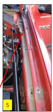
9. Place one 90 deg bracket on the exposed inner fender, so that the side of the bracket is against the inner fender, and the back of the bracket rests against the reinforced (raised) portion of the inner fender (red arrows) (**Fig 6**).
