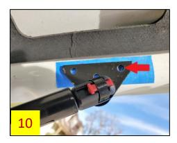
NOTE: The location of the bracket along the length of the hood may be different from these pictures, depending on the chosen hood height. To answer a question we sometimes get, no measurements are needed for locating the bracket – as long as the hood is at the desired position during bracket installation, simply install the bracket where it meets the hood when the strut is raised, as stated in Steps 13-14.
