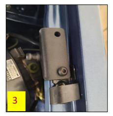
9. Insert another supplied M6 x 1.0 x 16 mm bolt into the rear hole in the bracket, and thread a supplied M6 x 1.0 nut onto the back side of the bolt (Fig 4).
