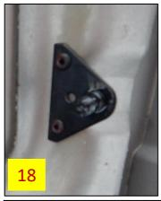
22. If you removed the strut from the bracket in Step 20, place the strut tube end fitting back onto the bracket. Push the spring clip on the back of the fitting into place (**Fig 19**).
