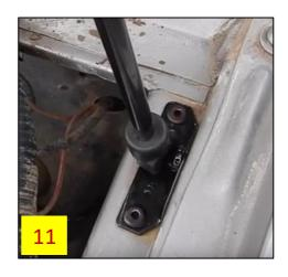
**NOTE**: Do **NOT** push the tube end fitting of the strut (with the SPIKER sticker) onto the fender ball bracket. See **Fig 12** for correct strut orientation.
