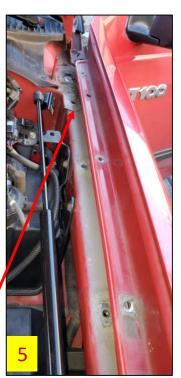
9. Place one 90 deg bracket on the exposed inner fender, such that the side of the bracket is against the inner fender, and the back of the bracket rests against the reinforced (raised) portion of the inner fender (red arrows) (**Fig 6**).
