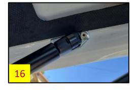
23. Remove the strut from the flat bracket to gain access for drilling the second hole. To disconnect the strut from the bracket, use a flat blade screwdriver to lift the semi-circular clip at the back of the fitting, until the fitting can be removed from the bracket (Fig 17). Do not fully remove the clip.
