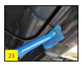
23. Line up the bracket hole with the drilled hole, and use a 3/16" rivet to attach the bracket (Fig 24). You may have to remove the strut from the bracket to gain access for rivet installation (see step 30).
