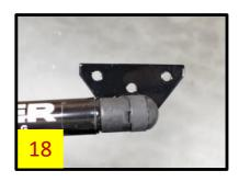
18. Raise the strut and flat bracket up until the bracket meets the inner side of the hood reinforcement (facing the center of the truck, NOT the outside) (Fig 19 & 20). The bracket should be just below the inside corner, flat against the reinforcement.
