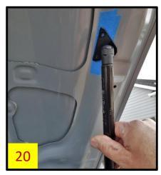
19. Apply some painter's tape to the hood reinforcement behind the bracket, and mark the location of the front hole with a permanent marker (red arrow in Fig 21 & 22). Lower the strut and bracket, and center punch the marked location.
