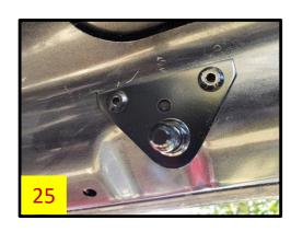
25. If you removed the strut from the bracket in Step 23, push the strut tube end fitting back onto the bracket. Push the spring clip on the back of the fitting into place (Fig 26).
