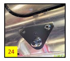
24. Make sure that the bracket is parallel to the hood frame. Using the bracket as a guide, drill the second hole, and install the second rivet to complete the bracket installation (Fig 25).
