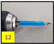
11. Drill two holes at the marked locations through the inner fender, using a slow speed and steady pressure on the bit (Fig 13). Apply WD-40 as needed to cool the bit. Remove the tape. Touch up the drilled holes with primer and paint.
