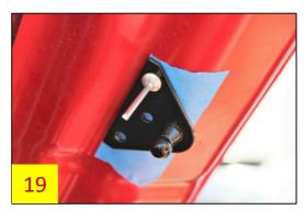
22. Adjust the bracket to be parallel with the hood frame. Using the bracket as a guide, drill the second hole and install the second rivet to complete the bracket installation (Fig 20).
