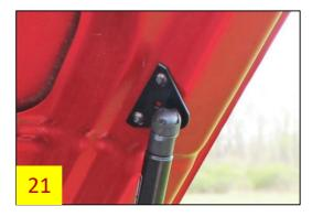
24. Repeat steps 16 through 23 for the passenger side. Do NOT assume that the location of the passenger side hood bracket will be identical to the driver side. Instead of measuring, use the same procedure for installing the bracket on the passenger side as you did for the driver side.
